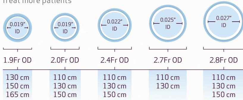
ID = Inner Diameter; OD = Outer Diameter; Diameter graphics not to scale
